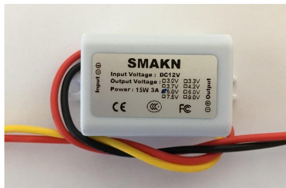
5VDC Voltage Regulator Required for reader power (see below) Pre-installed inside controller enclosure
