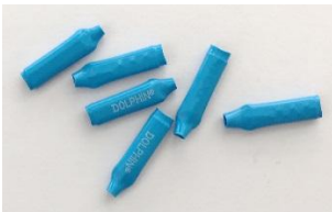
Crimp Connectors (Found in controller enclosure)
